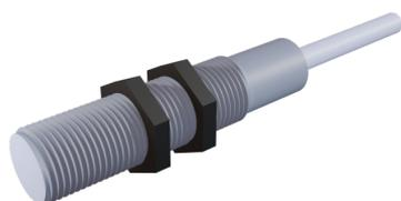
**SENSOR CAPACITIVO DIAMETRO 12mm LARGO 59mm RAS Sn = 1-3mm 10-30Vdc NPN NA 100Hz PLASTICO CABLE 2m**
