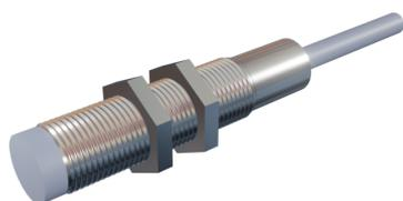
**SENSOR CAPACITIVO DIAMETRO 12mm LARGO 59mm Sn = 1-6mm 10-30Vdc PNP NC 100Hz CABLE 2m**
