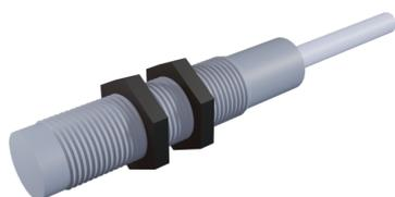
**SENSOR CAPACITIVO DIAMETRO 12mm LARGO 59mm Sn = 1-6mm 10-30Vdc PNP NA 100Hz PLASTICO CABLE 2m**
