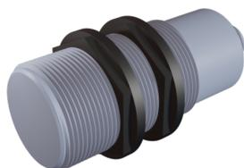
**SENSOR CAPACITIVO DIÁMETRO 30mm LARGO 80mm RAS Sn = 2-20mm 20-240Vac NC 25Hz PLASTICO CONECTOR M12**
