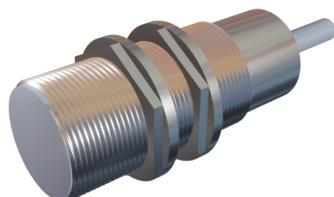
**SENSOR CAPACITIVO DIAMETRO 30mm LARGO 80mm RAS Sn = 2-20mm 10-30Vdc PNP NA+NC 100Hz CABLE 2m**
