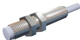
**SENSOR INDUCTIVO DIAMETRO 8mm LARGO 45mm Sn = 2mm 10-30Vdc NPN NA 1000Hz CABLE 2m**
