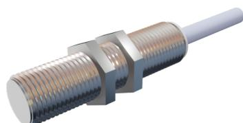
**SENSOR INDUCTIVO DIAMETRO 12mm LARGO 50mm RAS Sn = 2mm 20-250Vac/dc NA 25Hz AC, 40 Hz DC CABLE 2m METAL FACE**
