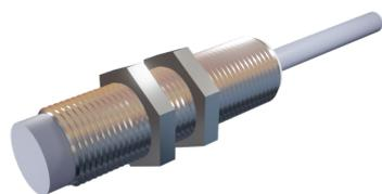
**SENSOR INDUCTIVO DIAMETRO 12mm LARGO 50mm S<sub>n</sub> = 8mm 10-30Vdc PNP NA+NC 500Hz CABLE 2m**
