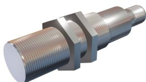
**SENSOR INDUCTIVO DIAMETRO 18mm LARGO 79mm RAS S<sub>n</sub> = 5mm 20-250Vac/dc NC 25Hz AC,40Hz DC 25Hz AC,40Hz DC CONE**
