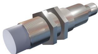
**SENSOR INDUCTIVO DIAMETRO 18mm LARGO 79mm S<sub>n</sub> = 0-7mm 4-20mA 18-30Vdc ANALOGO 500Hz CONECTOR M12**
