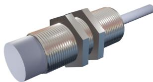
**SENSOR INDUCTIVO DIAMETRO 18mm LARGO 55mm S<sub>n</sub> = 8mm 20-250Vac NC 50Hz CABLE 2m**
