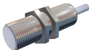
**SENSOR INDUCTIVO DIAMETRO 18mm LARGO 55mm RAS S<sub>n</sub> = 8mm 20-250Vac/dc NC 25Hz AC,40Hz DC CABLE 2m**
