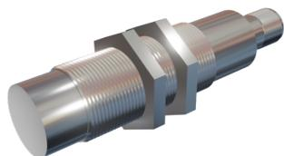
**SENSOR INDUCTIVO DIAMETRO 18mm LARGO 79mm S<sub>n</sub> = 10mm 10-30Vdc PNP NA 300Hz CONECTOR M12 METAL FACE**
