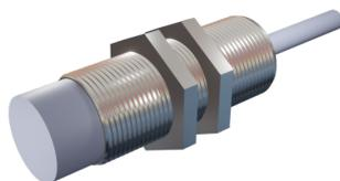
**SENSOR INDUCTIVO DIAMETRO 18mm LARGO 55mm S<sub>n</sub> = 16mm 10-30Vdc NPN NA+NC 150Hz CABLE 2m**
