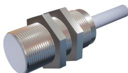
**SENSOR INDUCTIVO DIAMETRO 18mm LARGO 35mm CORTO RAS Sn = 8mm 10-30Vdc NPN NA+NC 500Hz CABLE 2m**
