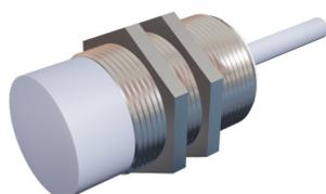
**SENSOR INDUCTIVO DIAMETRO 30mm LARGO 55mm S<sub>n</sub> = 15mm 10-30Vdc NPN NA+NC 150Hz CABLE 2m**
