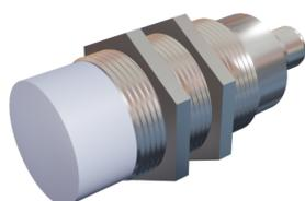
**SENSOR INDUCTIVO DIAMETRO 30mm LARGO 78mm S<sub>n</sub> = 15mm 20-250Vac/dc NA 25Hz AC,40Hz DC CONECTOR M12**
