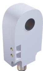
**SENSOR INDUCTIVO ANILLO 35x60x20mm S<sub>n</sub> = 10mm 10-30Vdc PNP NC 2000Hz CONECTOR M12**
