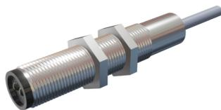
**SENSOR OPTICO DIAMETRO 12mm LARGO 67mm Sn = 0-5.2m BARRERA 10-30Vdc NPN NA 200Hz CABLE 2m**
