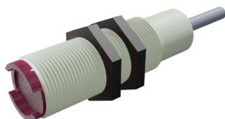
**SENSOR OPTICO DIAMETRO 18mm LARGO 78mm Sn = 0-3m REFLEX 24-240Vac NA 100Hz PLASTICO CABLE 2m**
