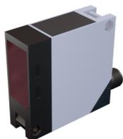
**SENSOR OPTICO 50x50x18 Sn = 0-10m REFLEX 20-250Vac/DC NA+NC 100Hz CONECTOR M12 GIRABLE**
