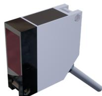
**SENSOR OPTICO 50x50x18 Sn = 0-20m BARRERA 10-30vDC PNP/NPN NA/NC 200Hz CABLE 2m**
